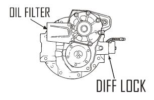
PUMP AND LOCK 2 AIR LINES TO UNIT
